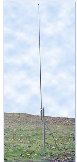
Figure 2. Clifton Laboratories Z1501F Voltage Probe Active Antenna (Antenna length = 10 feet)
