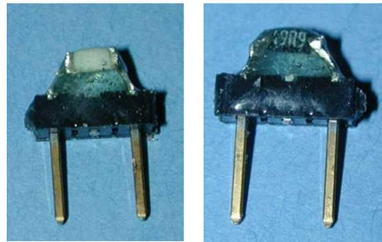
The result will be fragile; the resistor's ceramic substrate is easily broken. I use a small bit of 5-minute epoxy to encapsulate the resistor and mount to reduce the risk of breakage. In making crystal parameter measurements, it's generally good practice to ground the crystal case. I've added pads to solder two ground wires to that may be used to ground the crystal holder.
