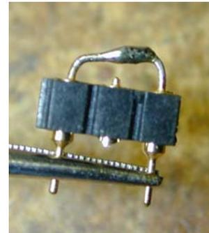
When working with the headers, the pins will sometime work loose if overheated, so you may find it helpful to hold the free ends with a heatsink clip, or a bit of wet tissue paper may be placed on them. Alternatively, you may be able to bend the solder-side of the pins until nearly touching and bridge the gap with solder. The header assemblies are fragile and I prefer to use the foil for mechanical reasons.
