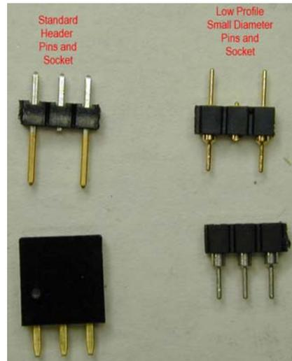
The standard header socket will work with HC-49 crystal leads, but the connection will not be nearly as solid as with the smaller socket. ¼ watt resistor leads and many small capacitor leads will fit the standard socket, which extends the usefulness of the fixture.
