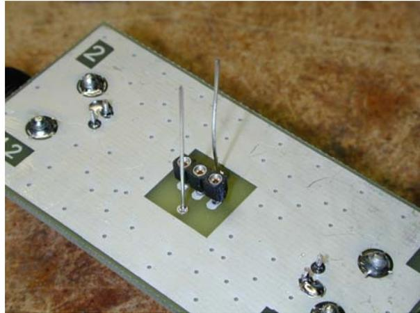
Install two solid wires, approximately 1 inch (25 mm) extending above the PCB surface as illustrated.
